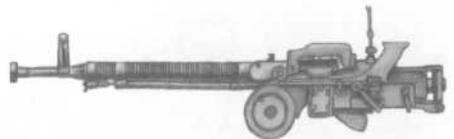
Introduced in 1969, the NSV is a heavy machinegun that has slowly been replacing the DShKM, above. It is a gas-operated weapon firing the same round as its predecessor. It is essentially the same in features and use, but is substantially lighter and features a quick-change barrel.
