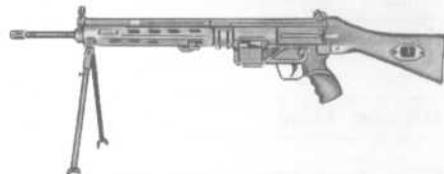
Derived through a long evolution from the G33 assault rifle, the 23E is a 5.56mm light machinegun. It is blowback-operated, firing from the open bolt and using the roller-locked bolt mechanism. It features a bipod, quick-change barrel, and selective fire that allows single shots, three-round bursts, and automatic fire. The 23E is belt-fed, accepting continuous- or disintegrating-link belts.
