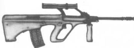
An unusual and exotic-looking weapon, the AUG (Armee Universal Gewehr) is a bullpup assault rifle firing the 5.56mm round. It is ergonomically designed, and has modular components allowing it to be converted to a light machinegun, a submachinegun, and a shorter carbine version, by simply changing barrels and breech mechanisms. All of the AUG weapons are covered in this text (see pages 76 and 134).
